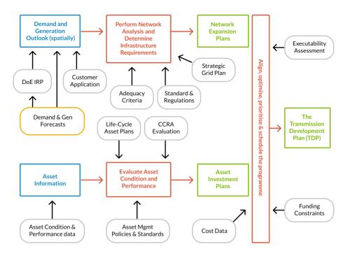
Figure 9.2: Graphical illustration of the planning process. The figure is adapted from the process employed by Chile
