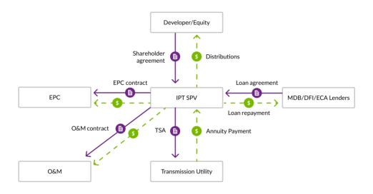
Figure 5.1: Relationship structure in an Independent Power Transmission Special Purpose Vehicle model
